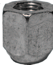
Chrome Open M12 x 1.50 Hex: 19mm Length: 21mm Seat: 60° Solid Steel
