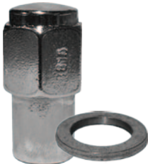
Chrome With Washer 1/2 - 20 Hex: 13/16 Length: 1.68 Seat: MAG Solid Steel
