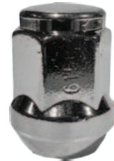
Chrome Acorn M12 x 1.50 Hex: 19mm Length: 32mm Seat: 60° Solid Steel
