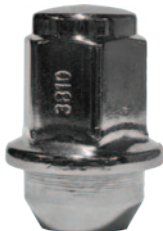
Chrome Acorn M14 x 1.50 Hex: 21mm Length: 43mm Seat: 60° Solid Steel
