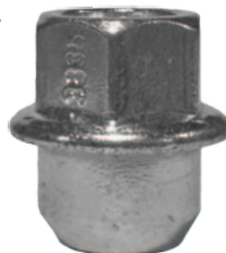
Zinc Retainer Open 1/2 - 20 Hex: 13/16 Length: 1.19 Seat: 60° Solid Steel
