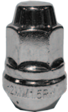
Chrome Acorn M12 x 1.50 RH Hex: 17mm Length: 35mm Seat: 60° Solid Steel
