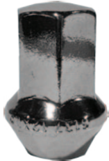
Chrome Acorn M12 x 1.50 Hex: 19mm Length: 38mm Seat: 60° Solid Steel
