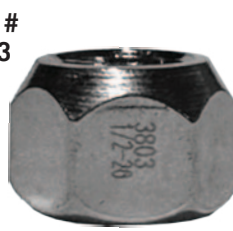
Zinc Open 1/2 - 20 Hex: 3/4 Length: 0.56 Seat: 60° Solid Steel
