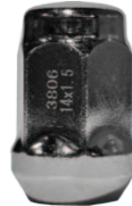
Chrome Acorn M14 x 1.50 Hex: 19mm Length: 35mm Seat: 60° Solid Steel
