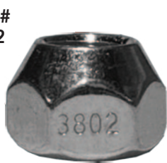
Zinc Open 1/2 - 20 Hex: 13/16 Length: 0.66 Seat: 60° Solid Steel
