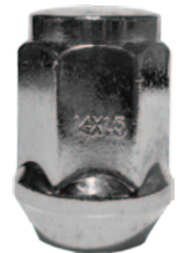
Chrome Acorn M14 x 1.50 Hex: 21mm Length: 36mm Seat: 60° Solid Steel
