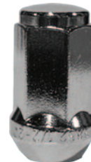
Chrome Acorn Dome Top 1/2 - 20 Hex: 3/4 Length: 1.60 Seat: 60° Solid Steel
