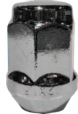
Chrome Acorn M12 x 1.50 Hex: 21mm Length: 32mm Seat: 60° Solid Steel
