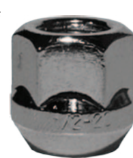
Chrome Open Bulge 1/2 - 20 Hex: 3/4 Length: 0.84 Seat: 60° Solid Steel
