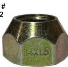
Zinc Open M14 x 1.50 Hex: 22mm Length: 16mm Seat: 60° Solid Steel
